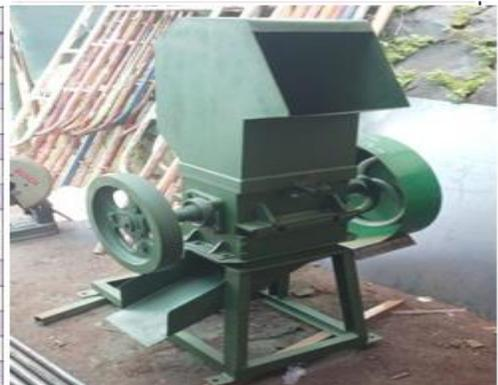
**Gambar 6. Detail Mesin SHREDDING (HY500)**
