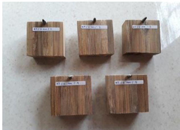
Gambar 5.26 Uji Tumpu Sekrup Cut Thread Wood (CTW)
