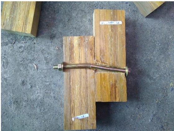
Gambar L-5.3. KS-8mm-3 (Mode Kegagalan IIIIm)
