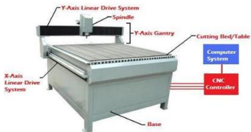
Gambar 2-3 bagian-bagian CNC Router
