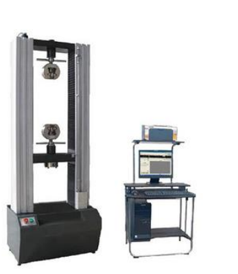
Gambar 2.3 Safety belt tensile strength test machine
