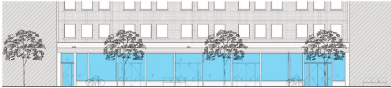
MINIMUM 70% CLEAR GLAZING BETWEEN 2 AND 10 FEET
