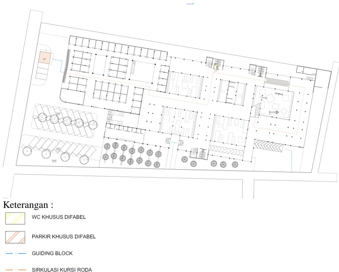
**Gambar 4. 20** Skema Barrier free Design
