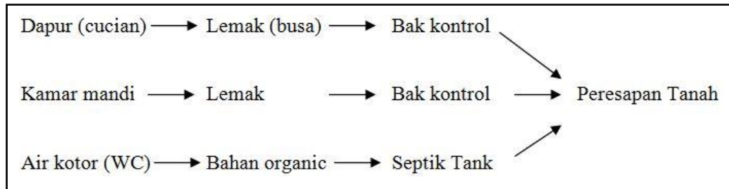
Gambar 4. 8 Skema distribusi air kotor
