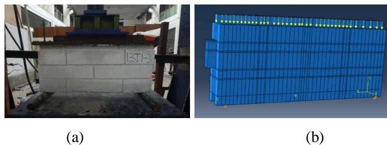
Gambar 4.8 (a) Eksperiment Setup In Plane , (b) Pemodelan In Plane
