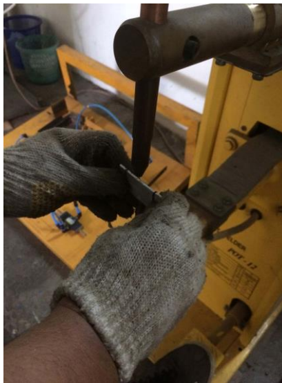
Gambar 3-9 Proses penyambungan plat pewter metode resistance soldering
