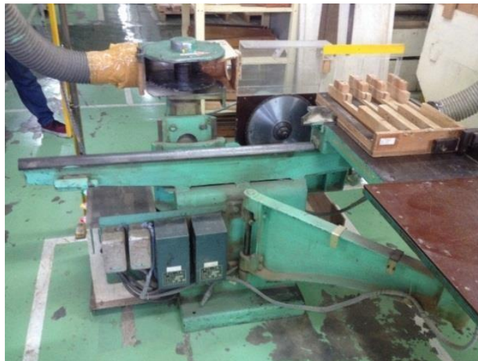
Gambar 2.3. Single Tenoner di PT. Yamaha Indonesia
