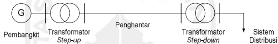
Gambar 2. 2 Single Line Diagram
