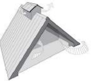
Gambar 2.21 Roof Venting. Sumber: jeffe dkk., 2020.
