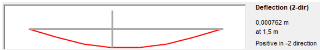
Gambar 5.52 Hasil Pengecekan Lendutan Batang L 100x100 Horizontal
