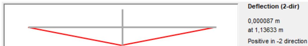
Gambar 5.56 Hasil Pengecekan Lendutan Batang L 100x100 Diagonal
