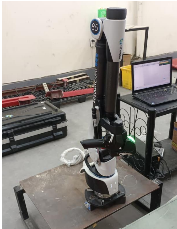
Gambar 3. 6 Hexagon 3D Scanner
