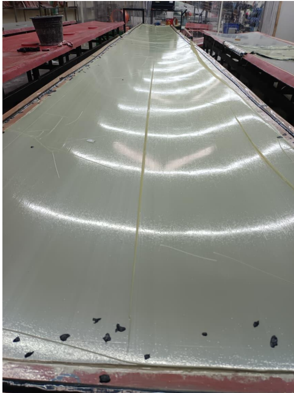
Gambar 3. 2 mold Wing Box Upper Skin Panel
