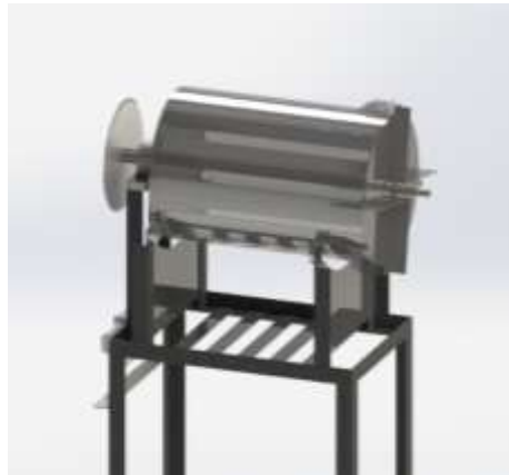
Gambar 4-1 Rancangan pertama rotary kiln reactor skala laboratorium
