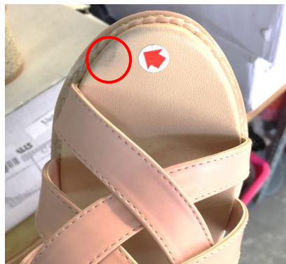
Gambar 5.3 Contoh Cacat Noda Lem
