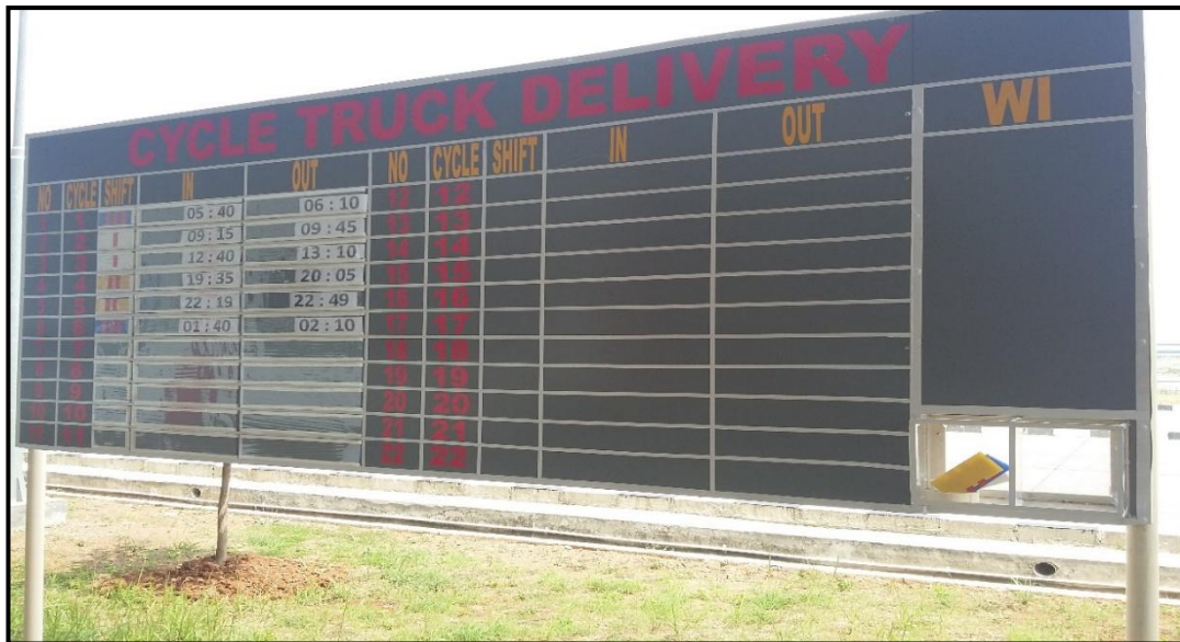
Gambar 5.18. Hasil Perancangan Papan Kedatangan Truck Delivery New Plant 1B
