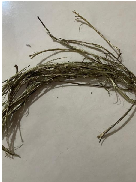
Gambar 4. 1 Serat Hasil Metode Water Retting
