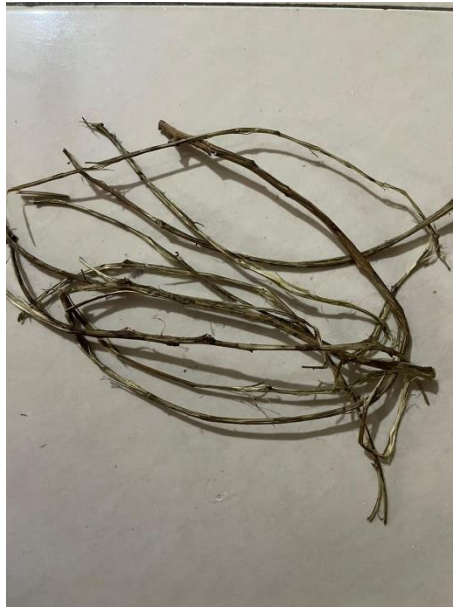
Gambar 4. 2 Serat Hasil Metode Manual Scraping
