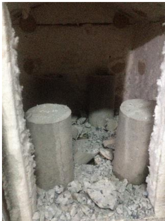
Gambar L-3.8 Beton Plastocrete ® RT6 Plus mengalami explosive spalling temperatur 700°C
