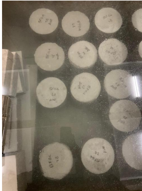
Gambar 7.3 Proses Perawatan Beton
