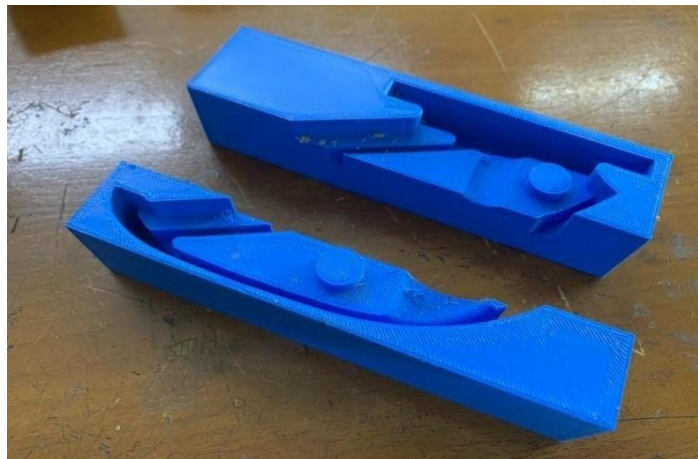
Gambar 4.13. Hasil 3D print JIG fixture .
