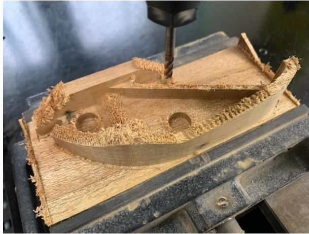
Gambar 4.14. Proses machining sisi-1.
