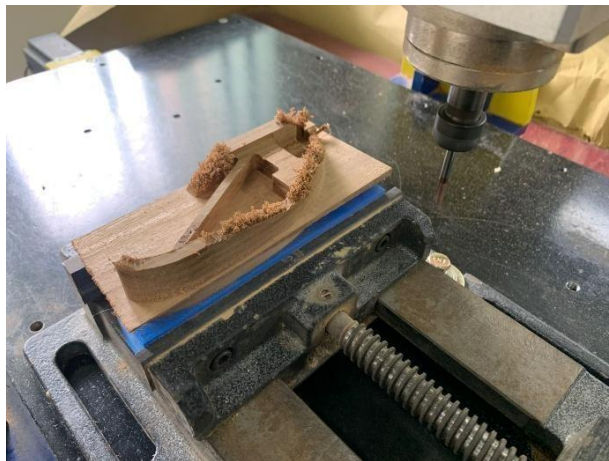
Gambar 4.15. Proses machining sisi-2.
