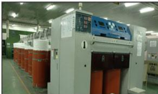
Gambar 4.6 Mesin Drawing Finisher
