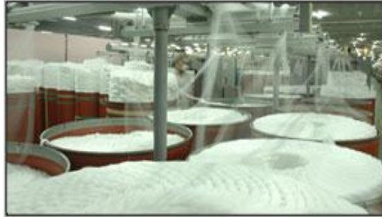
Gambar 4.5 Mesin Drawing Breaker
