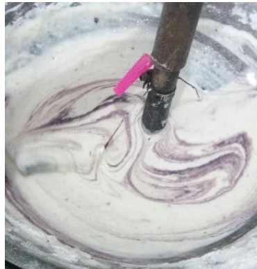
Gambar 4. 6 Uji prototype pengaduk jenis pitched blade paddle
