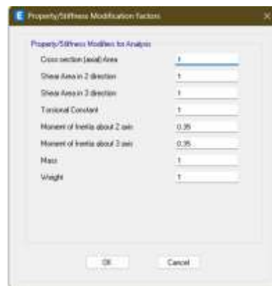
Gambar 5.18 Property/Stiffness Modification Factors Balok
