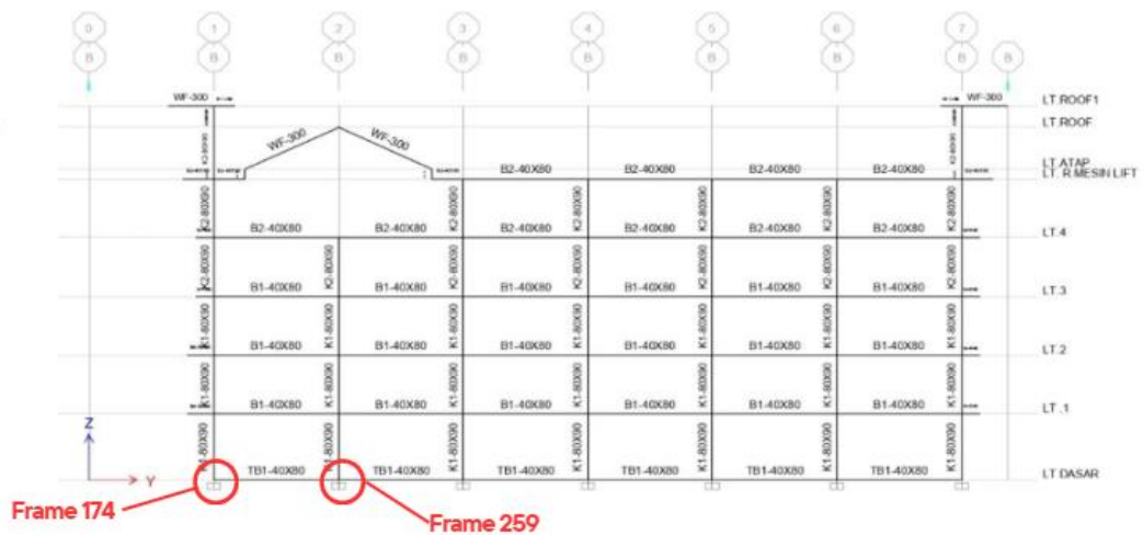
Gambar 5.7 Tampak - B Elevasi Samping Etabs
