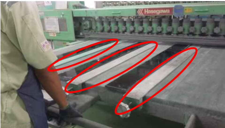
Gambar 5. Proses sanding permukaan mesin sanding #240 sesudah kaizen
