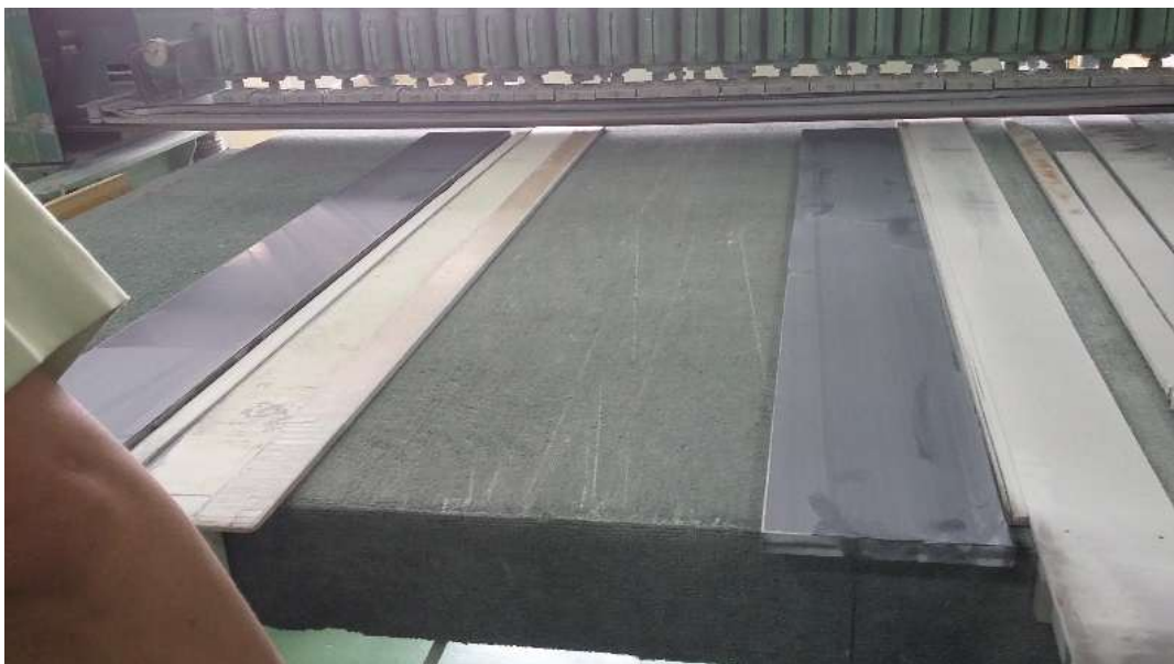
Gambar 9. Proses sanding permukaan mesin sanding #1000 sesudah kaizen
