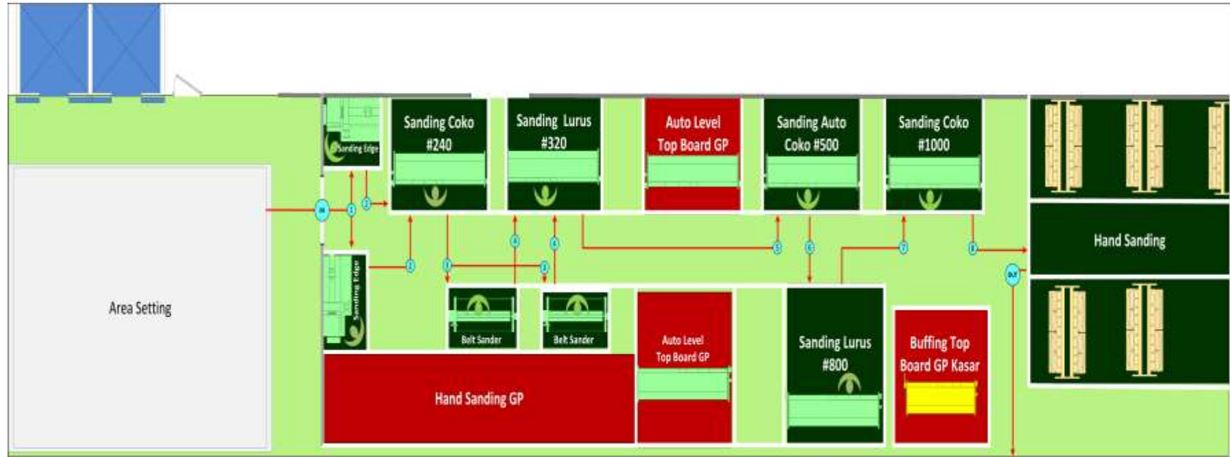
Gambar 1. Layout Sanding Panel UP
