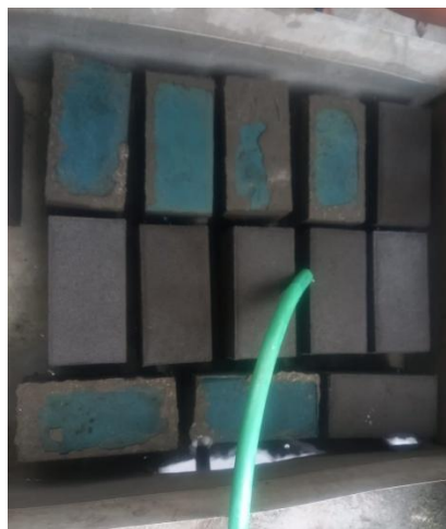
Gambar 4.29 Perendaman Paving Block
