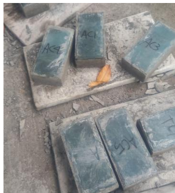
Gambar 4.28 Paving Berlapis Plastik
