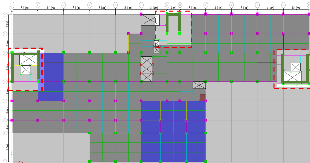
Gambar 5.4 Denah Dinding Geser Tipikal Lantai 1-7
