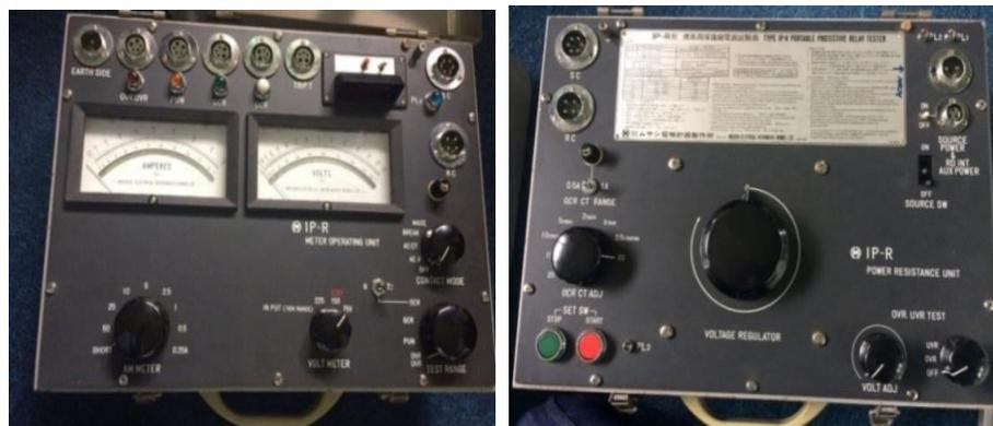
**Gambar 3.3** Portable relay tester tipe IP-R
