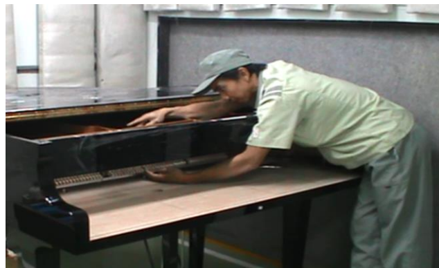
Gambar 4. 6 Proses Leveling of Damper
