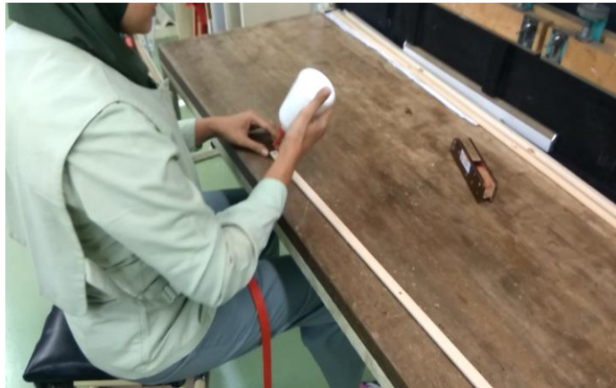
Gambar 4. 20 Pengeleman Key Front Rail
