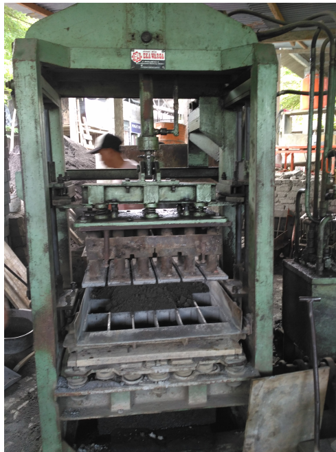
Gambar Proses Pencetakan Paving Block
