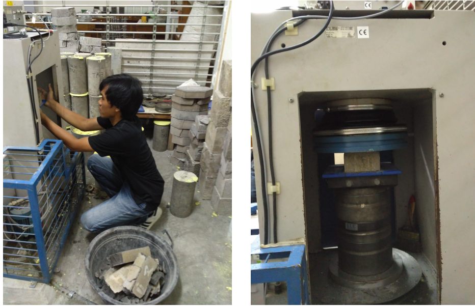
Gambar Proses Pengujian Kuat Desak Paving Block
