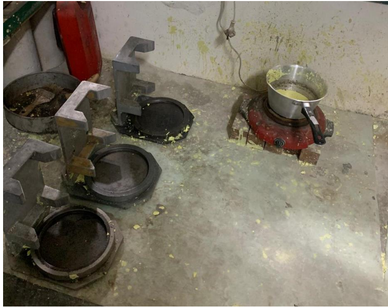
Gambar 6. 11 Peralatan Caping Silinder Beton
