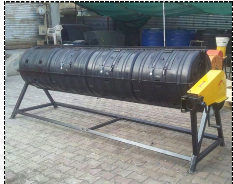
Gambar 2.63. Rotary Drum Composter Besar
