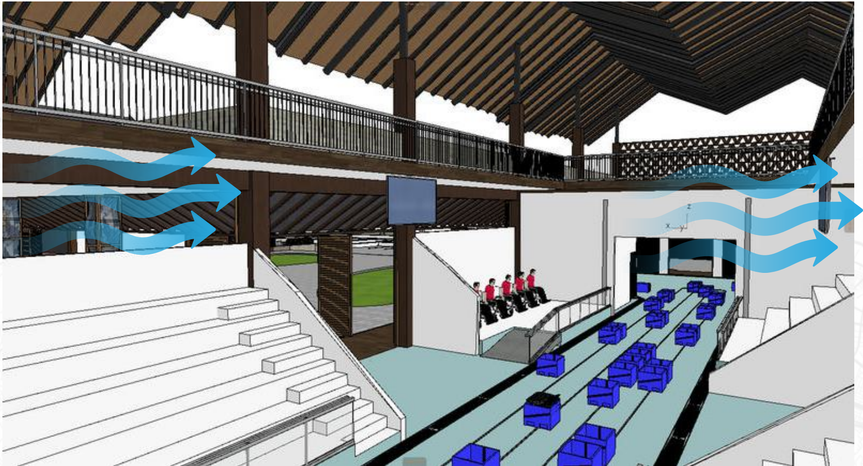
Gambar 3.22 Penerapan Konsep Open Building
