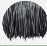
Palm Fiber additional material, used for the roof
