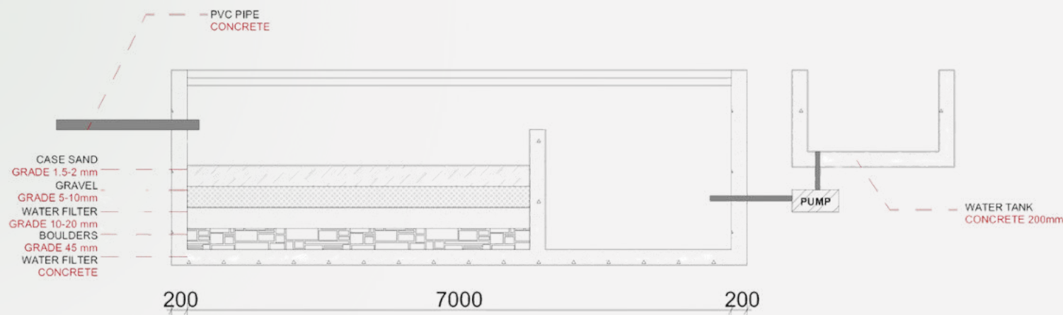
Figure 3.33 Water Harvesting System Detail (Author, 2025)
