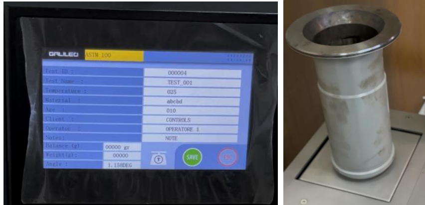
Gambar 4. 2 Proses Balancing Cetakan Gyratory
