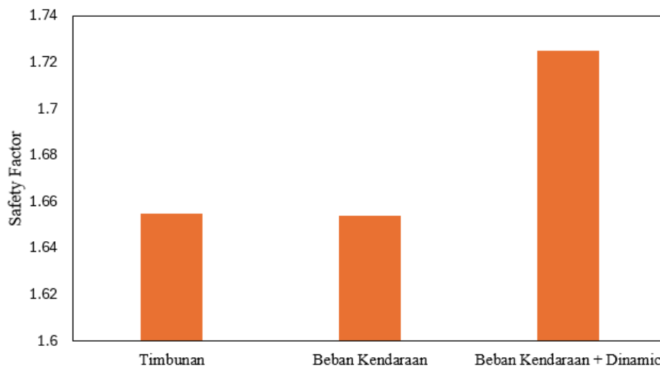
Gambar 6.14 Hasil Perhitungan Safety Factor Timbunan Tanah
