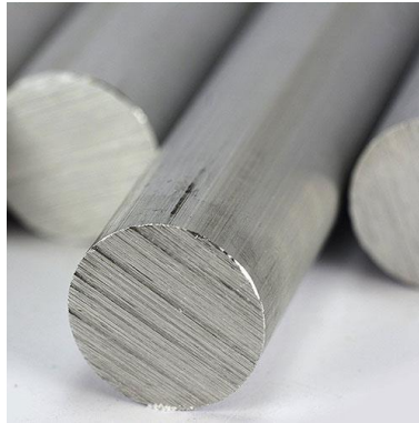
Gambar 3-45 As Aluminium Bulat OD 25mm
