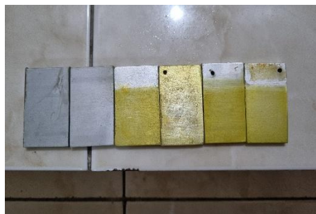
Gambar 4-6 Kegagalan Proses Anodizing
