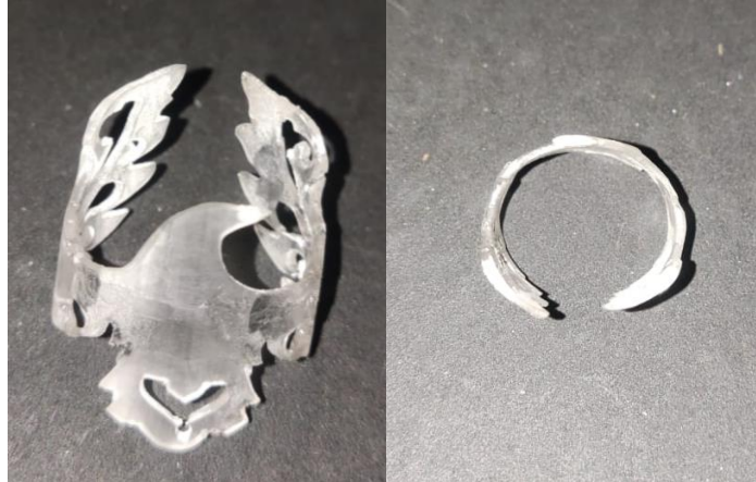
Gambar 4. 9 Hasil Master Cincin Garuda Relief
