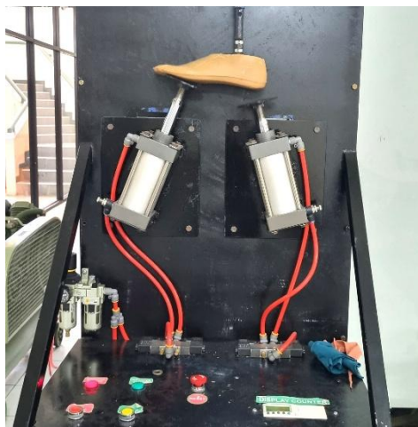
Gambar 4.23. Pengujian preliminary fatigue .
