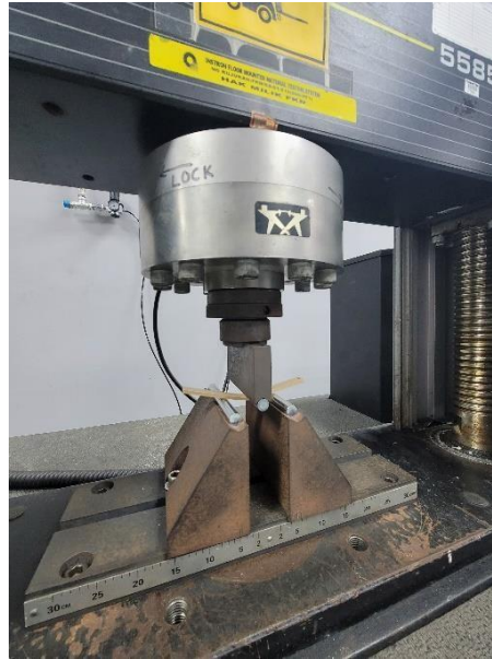
Figure 3-15 Placement of flexural specimen
