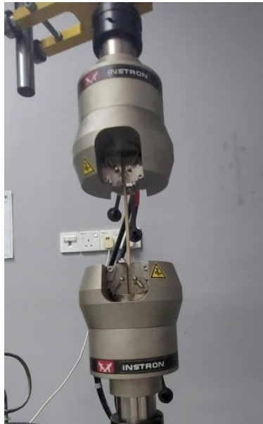
Figure 3-13 Placement of tensile specimen
