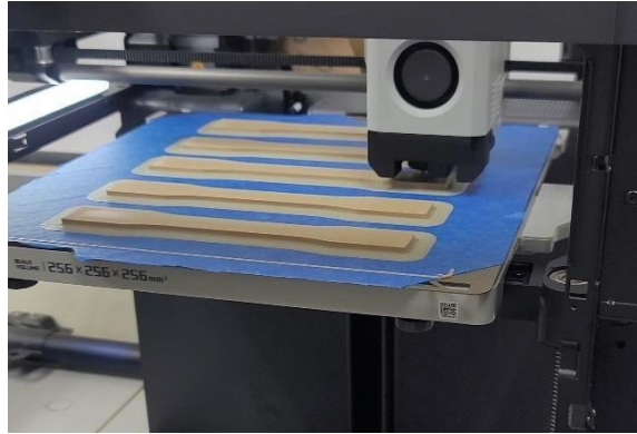
Figure 4-16 Brim and Blue tape applied
