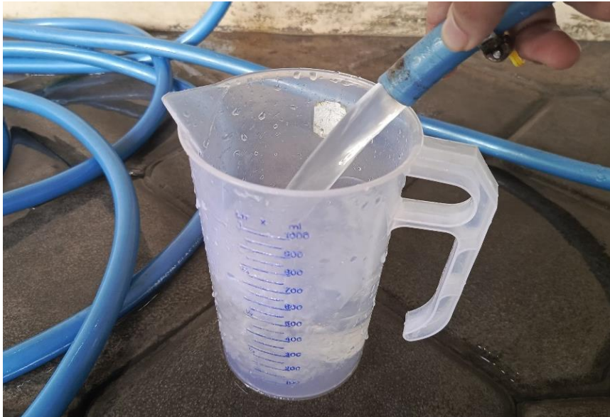
Gambar 4.22 Pengambilan sample debit air
