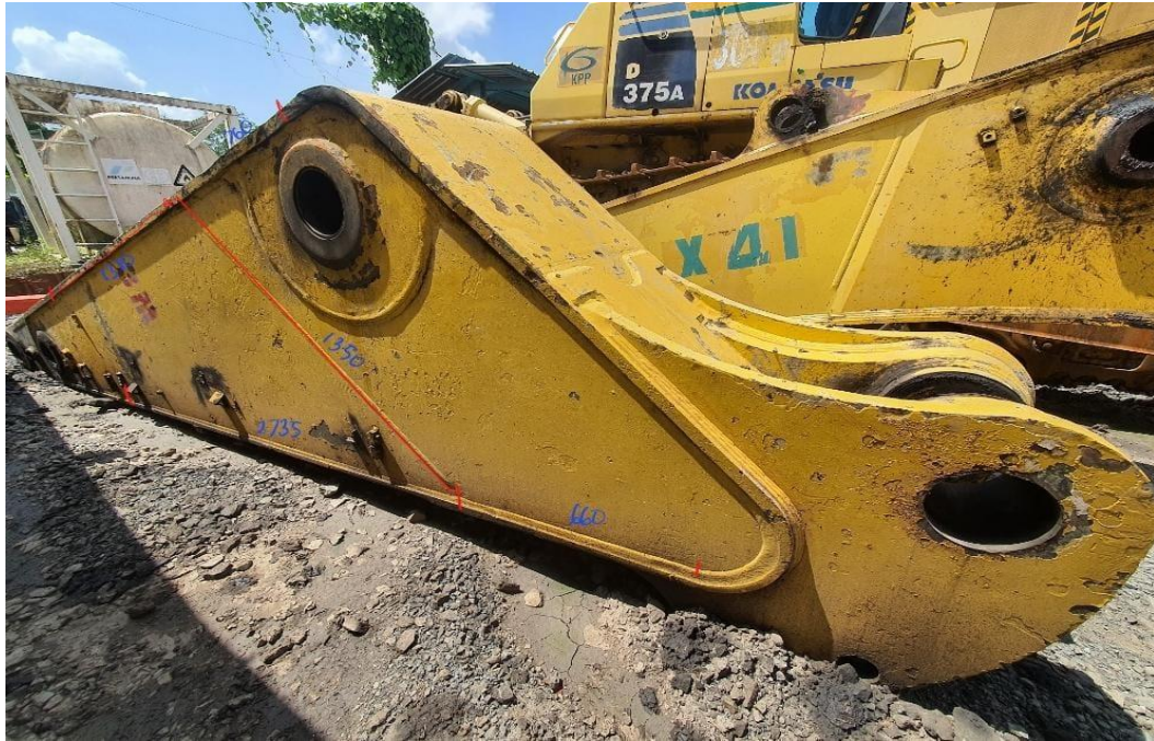
Gambar 3-3 Model 2D pengukuran arm Excavator Komatsu PC1250SP-11R
