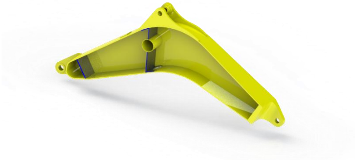
Gambar 4-2 Section view desain boom Excavator Komatsu PC1250SP-11R
