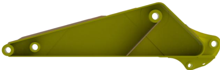
Gambar 4-4 Section view desain arm Excavator Komatsu PC1250SP-11R
