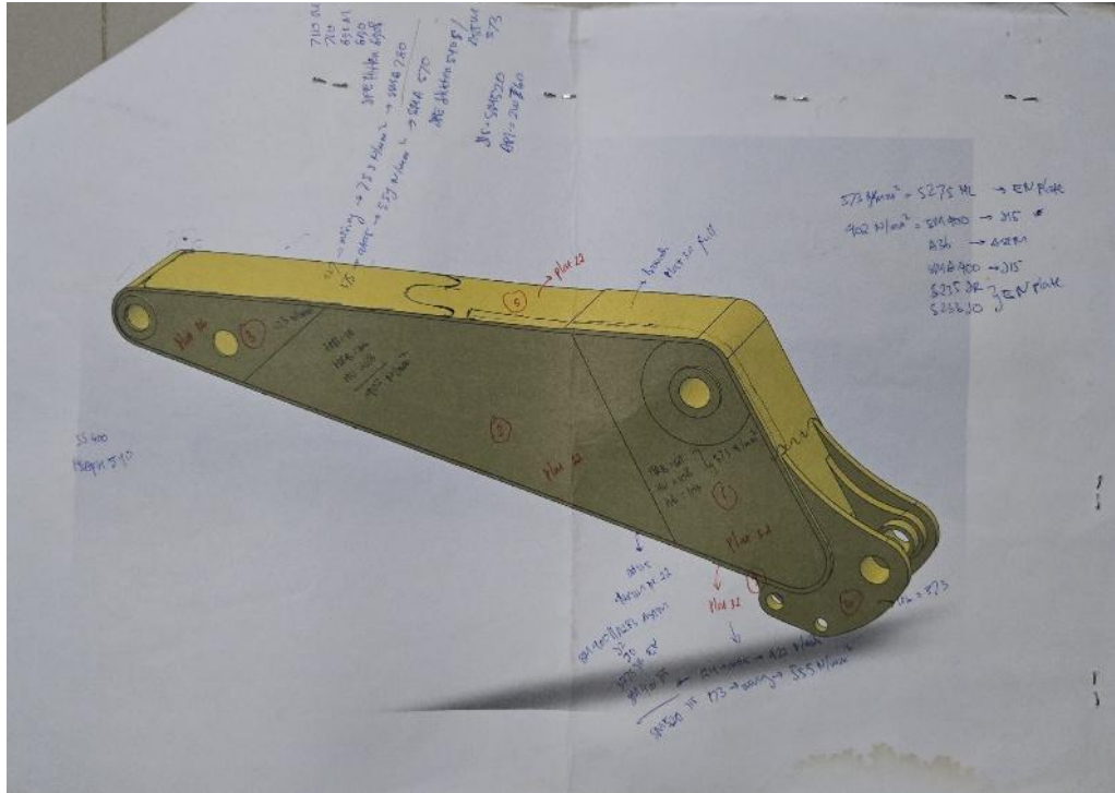
Gambar 3-5 Hasil pengukuran ketebalan arm Excavator Komatsu PC1250SP-11R
