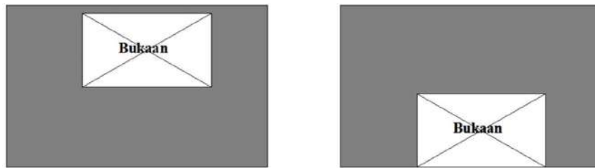
Figure 3.8 A Diaphragm Discontinuity Irregularity Illustration
