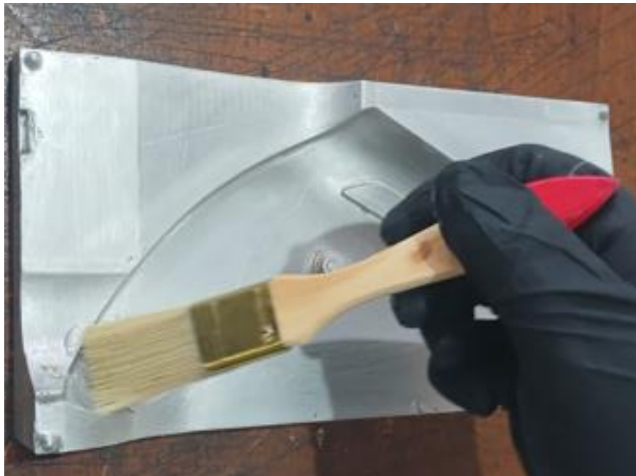
Gambar 3-6 Proses pelapisan wax mold release
