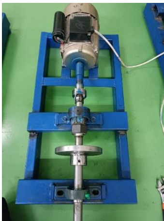
Gambar 3- 15 Pemasangan Housing Bearing Radial
