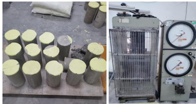
Figure 5. 20 Split Tensile Test Process
