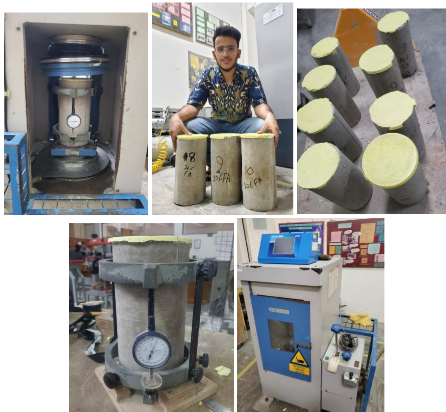
Figure 5. 22 Modulus of Elasticity
