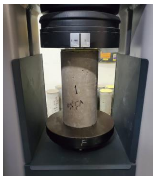
Figure 5. 18 Compressive Test Process
