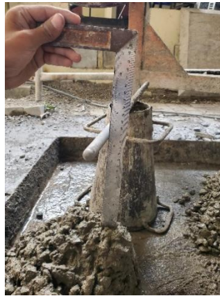
Figure 3. 1 Slump Test Using Abrams cone
