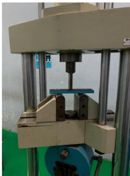
Gambar 4-1 Proses Pengujian Three Point Bending
